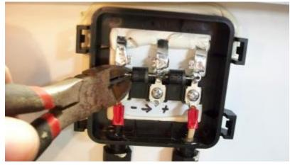
Loosen the 3 screws, and slip the replacement diodes in as shown. It is VERY IMPORTANT to orient the diodes properly. The silver stripe goes in the direction of the arrow. Snug the screws back up, being very careful not to strip the threads. Replace the cover and snap it into place
