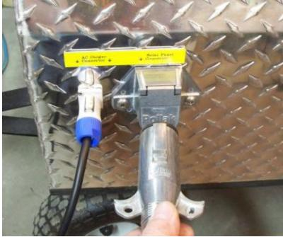
(Although both connectors are shown connected in the upper photo for illustration purposes, it is not recommended that both the AC charger and the solar charger operate at the same time.)
