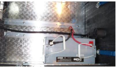
*Right;* The attachment point for the hinge-side battery strap is partially concealed by the soft-start module.
