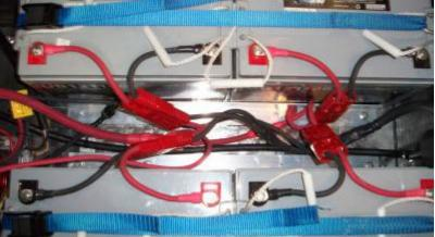
**Step 5**: *Right;* Disconnect the red connectors by pulling the two halves straight apart. Remove the batteries
