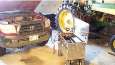
**Step 2:** Position the power station a comfortable distance from the vehicle, then, first, plug the cables into the power station, then affix the clamps to the vehicles battery.
