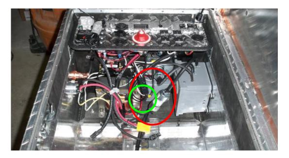
**Step 3:** *Right*, Remove the 4 screws on the hinge-side of the cabinet, and remove the soft-start module.
