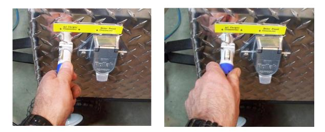
Insert the plug into the socket with the silver tab on top, and turned slightly to the left. Push it in fully and gently twist it clockwise until it latches. To remove, use your thumb to pull the silver tab toward you, then twist the plug counter-clockwise and pull it out of the socket.
