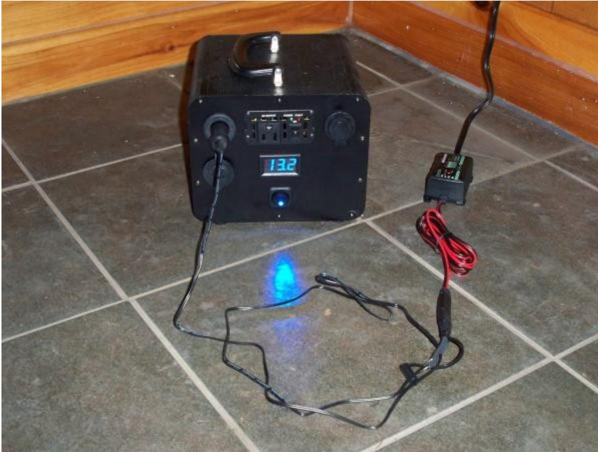
To recharge the unit when there is no sun, an optional AC charger is available. To use, plug the AC charger into a wall socket, and plug the cigarette-style plug into the DC receptacle as shown. The main switch must be on. The charger unit will display a red LED when charging, and when fully charged, the LED will turn green. The AC charger is fully automatic, so may be left plugged in with no harm even if the solar panel is also receiving sunlight.
